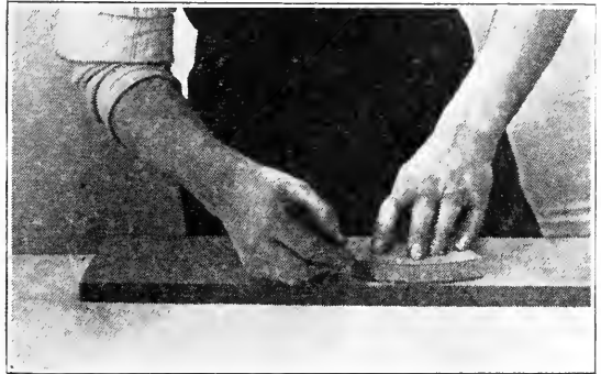
FIG. 551. LAYING OUT SEGMENTS.
